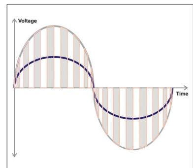
It has real benefits for incandescent lamps as it largely removes audible filament noise. However, it can be problematic with LED lamps - often causing flicker at the switch-on or switch-off points. Conclusion: Sine wave dimmers should be tested with your chosen LED lamps before committing.
