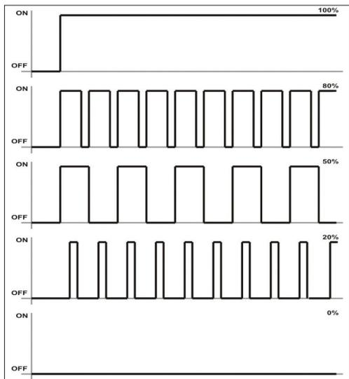
The frequency of modulation is not set by the mains frequency but is defined by the design. A PWM frequency of at least 1000Hz is required to ensure that no flicker is perceived. Conclusion: Check the modulation frequency is above 1KHz. Otherwise any flicker issues are likely to be related to the control (DMX / DALI / 0-10V) input.
