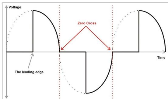
The SCR automatically switches off at the zero cross, so the percentage of the mains cycle between the leading edge and the zero cross defines the intensity of the lamp. This form of dimming actually causes the lamp to flash on and off at a frequency of 100Hz. When used with incandescent lamps, the eye's persistence of vision and the thermal inertia of the lamp mean that no flicker is perceived.
