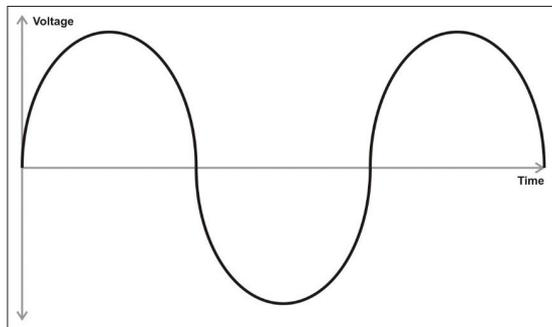
The first type of dimming used a technique called leading edge dimming. An electronic device called a Silicon Controlled Rectifier (SCR) is used to define the point in the AC waveform at which the power to the lamp is switched on (called the leading edge).
