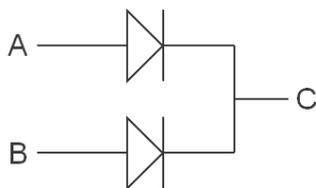
A represents an output from the first control console. B represents the second control console and C is the output which drives the dimmers (or moving lights or LED strips).
