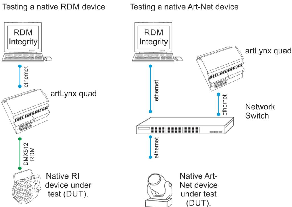
In this example the Artistic Licence gateway "artLynx quad" is used to route native RDM data from the DUT, to Integrity. It also operates as a dongle to unlock the RDM Integrity software.
